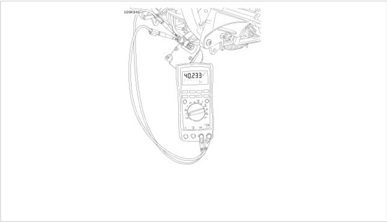
Figure 5. Check Stator AC Voltage Output (Typical)
