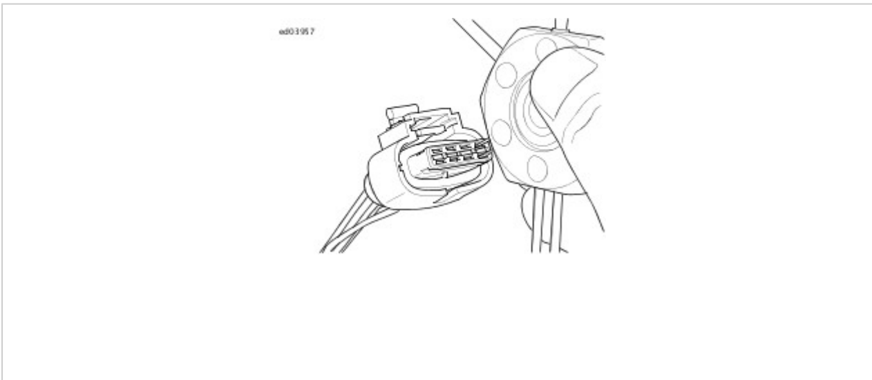
Figure 1. Terminal Removal: Bosch Compact 1.1M Connector
